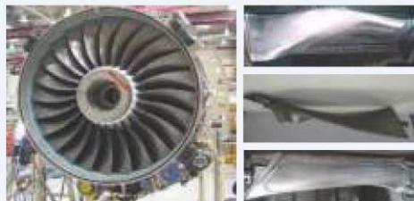
Blades: Weight: 5to25kgs. Mtrl: Ti alloys
